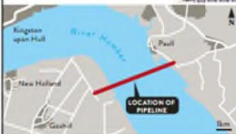
Between Goxhill and Paul on the River Humber, a slurry tunnel boring machine (TBM) known as *Mary* has dug a 5km-long tunnel.
